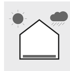
Panels should be stored in sheltered rooms
